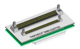
Another addition to the RAMCHECK® line provides a solution for testing older style 72-pin and optionally 30-pin standard EDO/FPM DRAM SIMM modules.
