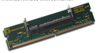
The RAMCHECK DDR2 200-Pin Converter (p/n INN-8668-12-1) is an inexpensive solution for testing modern laptop DDR2 memory. The converter plugs directly into the 240-pin RAMCHECK DDR2 main adapter (p/n INN-8668-12), providing you with fast, convenient testing capabilities for modern DDR2 SO-DIMM modules. Please note that you must have the DDR2 Adapter in order to use this converter.
