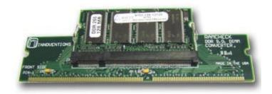
The RAMCHECK DDR 200-Pin Converter (p/n INN-8668-6-1) is an inexpensive solution for testing modern laptop DDR memory. The
