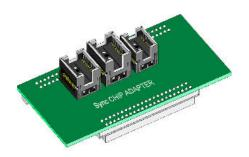
The RAMCHECK Sync CHIP Adapter supports popular TSOP chips in sizes of 16Mx16, 4Mx16, 32Mx8, 8Mx8, 64Mx4, 16Mx4 and more.
