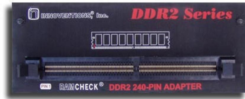
The RAMCHECK DDR2 240-Pin Adapter (p/n INN-8668-12) is for testing modern DDR2 DIMMs.
