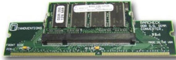
The converter is made in the shape of a standard 184-pin DIMM module, but without the center key. It has special electronics for RAMCHECK's auto-detection, and it is designed for low noise and short signal connections.
